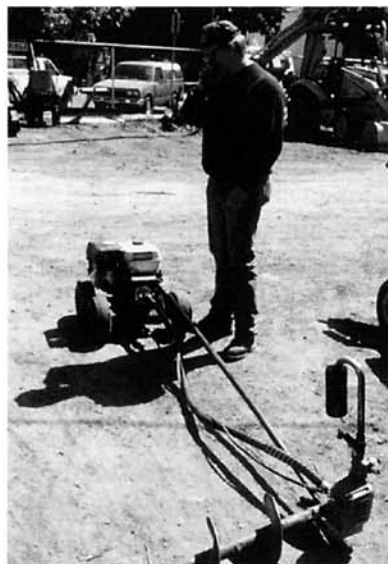
Heavy-duty commercial power augers that dig up to 12-inch holes 7 feet deep with add-on extensions are available from equipment rental shops.
