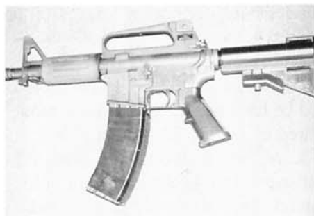
With its double 40-round magazine, this AR-15 pistol is virtually a crew-served handgun. The firepower is tremendous, and hits on target count for something.
