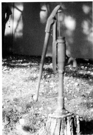
Some survivors with backyards can install their own shallow wells and old-fashioned hand pumps.
