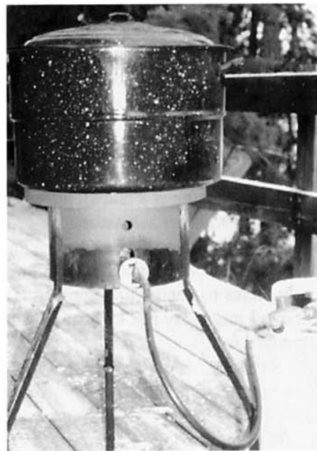
A home canning pot sits on a small, portable propane stove. Canning can be done virtually anywhere as long as supplies of LP gas hold out.
